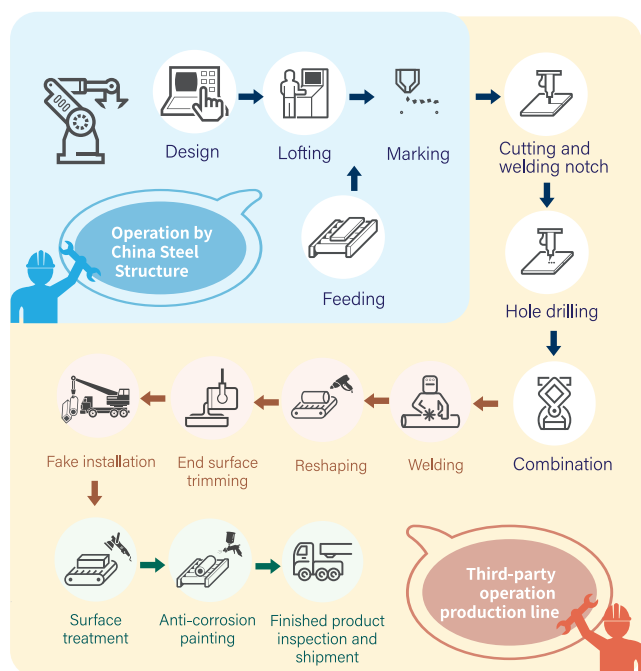
Steel Structure Manufacture Process Flow Chart
